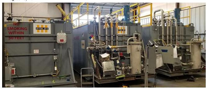
While the Covid-19 pandemic delayed many field installations, it did not delay the requirement to complete the products, systems, and equipment that would later be installed. Three 8,000 Gallon Fuel Systems are shown in different stages of production at Celtech's facility in Carlsbad, New Mexico.
